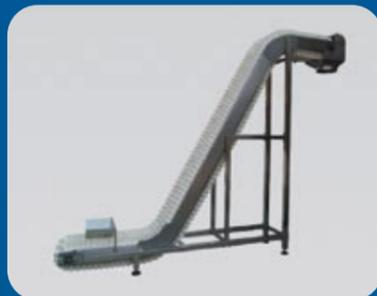
Inclined rubber belt conveyors
